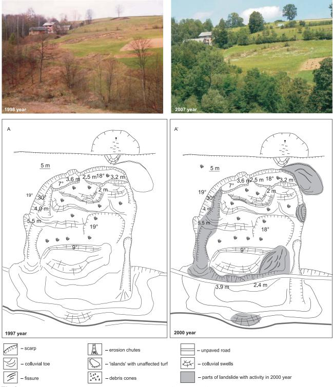
Fig. 2. A rotational slide on the slopes of the village of Młynne (form no. 966); A – map of the slide produced in 1997 immediately after it had occurred and before human intervention; A' – map of the same slide produced in 2000
