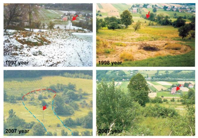
**Fig. 3.** Flow-slides (village of Laskowa, form no. 597); photos show the course of degradation of the toe section; the red arrow points to a reference point, a power line pole
