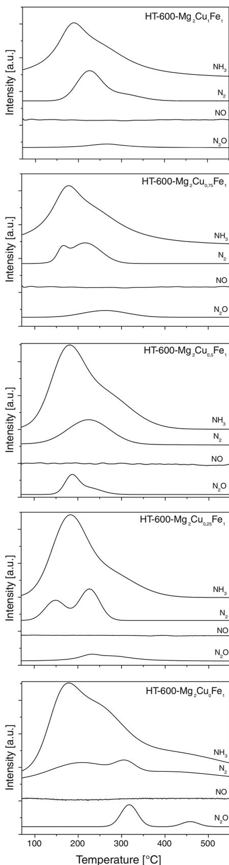
◀ Fig. 5 Results of temperature-programmed desorption of  $\text{NH}_3$  ( $\text{NH}_3$ -TPD) obtained for hydrotalcite derived catalysts. Conditions: 100 mg catalyst, adsorption: 70 °C, 1%  $\text{NH}_3$  diluted in He, flow rate = 20 mL/min, desorption: flow of pure He = 20 mL/min, linear heating rate of 10 °C/min
