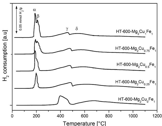
Fig. 2 Temperature-programmed reduction (TPRed) of mixed metal oxide catalysts. Conditions: 30 mg catalyst, 10% H<sub>2</sub> diluted in Ar, flow rate of 6 mL/min, linear heating rate of 5 °C/min
