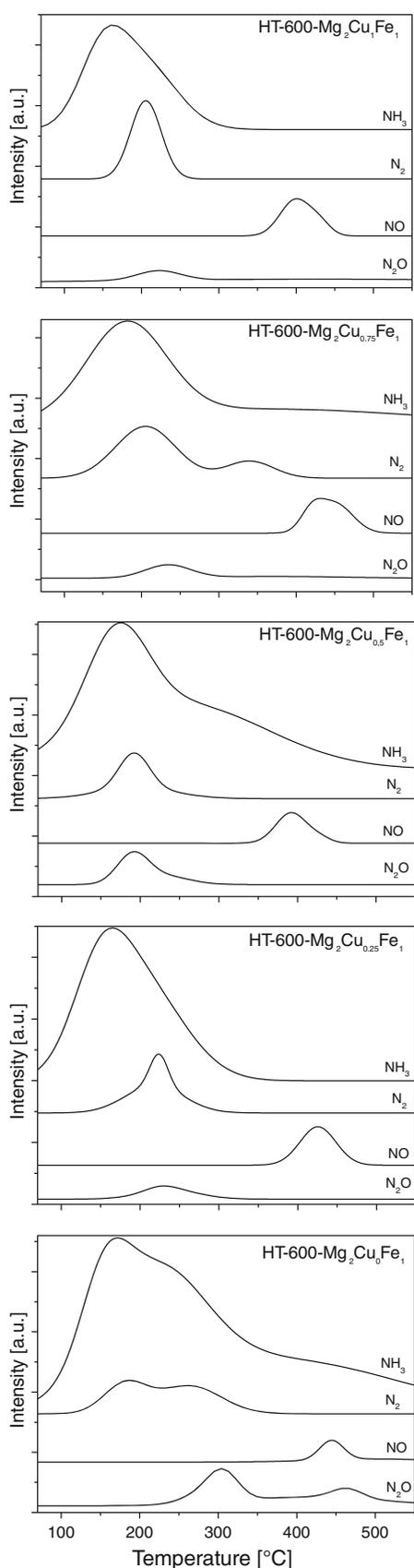
◀ Fig. 6 Results of temperature-programmed surface reaction ( $\text{NH}_3$ -TPSR) obtained for hydrotalcite derived catalysts. Conditions: 100 mg catalyst, adsorption: 70 °C, 1%  $\text{NH}_3$  diluted in He, flow rate = 20 mL/min, desorption: 5%  $\text{O}_2$  diluted in He, flow rate = 20 mL/min, linear heating rate of 10 °C/min
