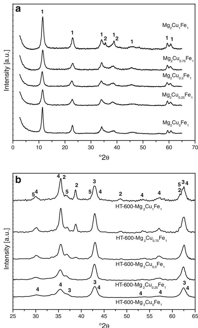
**Fig. 1** X-ray diffraction patterns for hydrotalcite-like catalysts' precursors (a) and mixed metal oxide catalysts (b); 1—hydrotalcite, 2—tenorite, CuO, 3—periclase, MgO, 4—magnesioferrite,  $\text{MgFe}_2\text{O}_4$ , 5—cuprite,  $\text{Cu}_2\text{O}$
