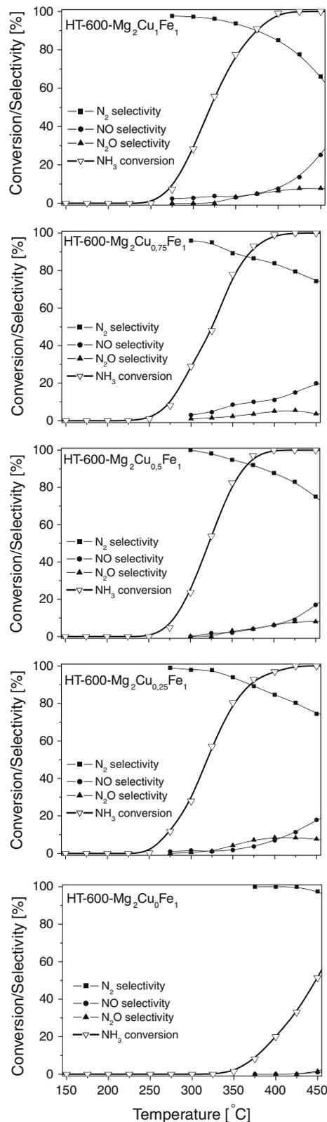
Fig. 3 Selective catalytic oxidation of ammonia over hydrotalcite derived catalysts. Conditions: 100 mg catalyst, [NH<sub>3</sub>] = 0.5%, [O<sub>2</sub>] = 2.5%, [He] = 97%, total flow rate = 40 mL/min
