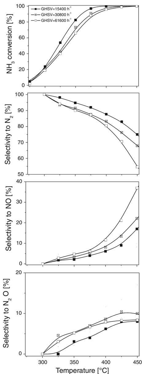
**Fig. 8** Effect of space velocity (SV) on activity and selectivity of HT-600-Mg<sub>2</sub>Cu<sub>0.5</sub>Fe<sub>1</sub> catalyst in the SCO process. Conditions: 25, 50 or 100 mg catalyst, [NH<sub>3</sub>] = 0.5%, [O<sub>2</sub>] = 2.5%, He = balance, total flow rate = 40 mL/min
