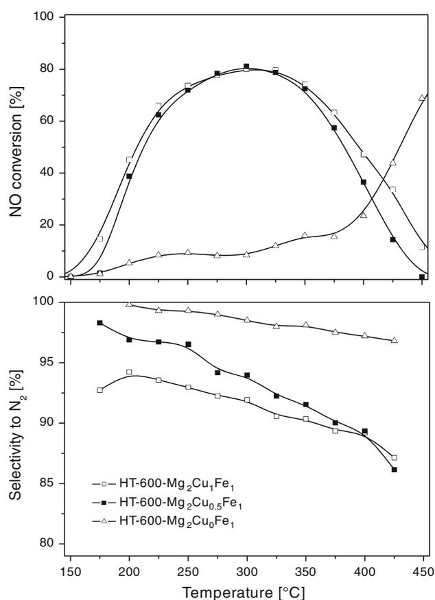
Fig. 7 Selective catalytic reduction of NO with ammonia over hydrotalcite derived catalysts. Conditions: 100 mg catalyst,  $[\text{NH}_3] = 0.25\%$ ,  $[\text{NO}] = 0.25\%$ ,  $[\text{O}_2] = 2.5\%$ ,  $[\text{He}] = 97\%$ , total flow rate = 40 mL/min
