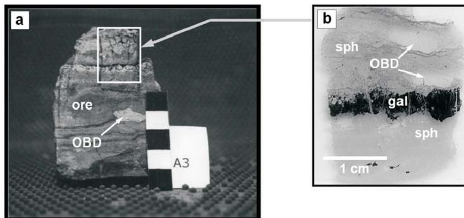
Fig. 2. (a) Sample taken from the boundary between the OBD and the ore body (scale – 5 cm).
