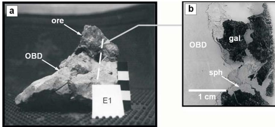
Fig. 1. (a) Sample taken from the boundary between the OBD and the ore body (scale – 5 cm).
