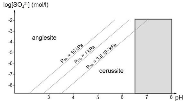
Fig. 6. Components that restrain solubility of Pb in solutions of different pH, different CO<sub>2</sub>(g) partial pressures and different amounts of SO<sub>4</sub><sup>2-</sup> represented as activity (mol/dm<sup>3</sup>). Modified after Reichert, Borg (2008). Grey rectangle represents pH conditions typical of a carbonate environment
