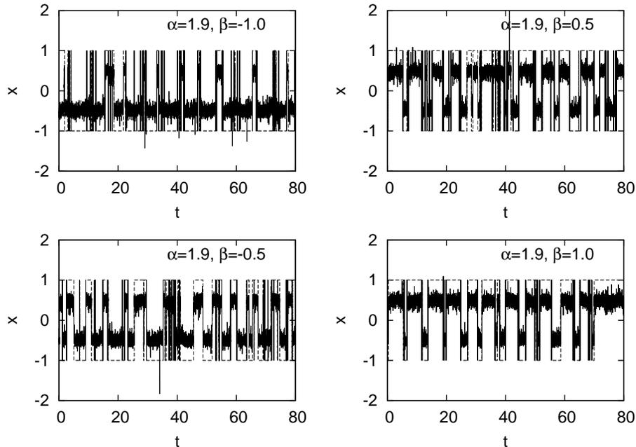
Fig. 4. Trajectories of an exemplary  $\alpha$ -stable processes constructed by use of Eq. (1) for a two-state approximation and for the full, continuous case. The two-state process takes values  $\pm 1$ . The time step of the integration is set to  $\Delta t = 10^{-5}$ , the scale parameter  $\sigma = \sqrt{2}$ . The frequency of a cycling voltage  $\Omega = 1$ . Noise parameters were chosen to examine possible effects coming from a skewness (bias) of the noise (see the text and *cf.* Fig. 3).
