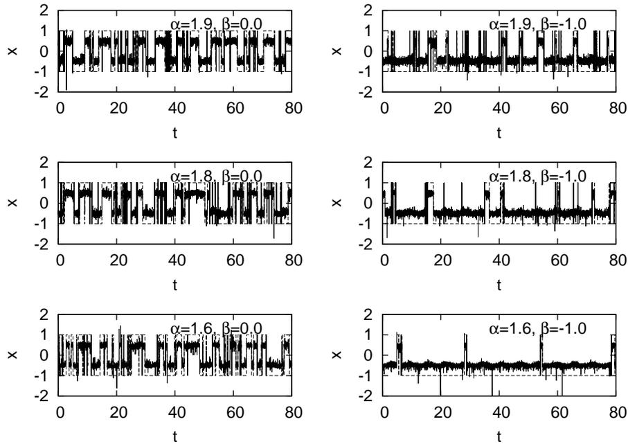
Fig. 7. Trajectories of the  $\alpha$ -stable processes for the two-state and the continuous model constructed by use of Eq. (1). The two state process takes values  $\pm 1$ . The time step of the integration  $\Delta t = 10^{-5}$ , the scale parameter  $\sigma = \sqrt{2}$ . The frequency of the cycling voltage  $\Omega = 1$ . Noise parameters as indicated in figures.
