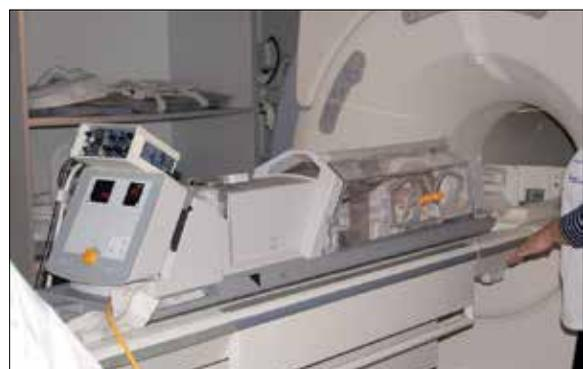
**Figure 1.** MR-compatible incubator.
