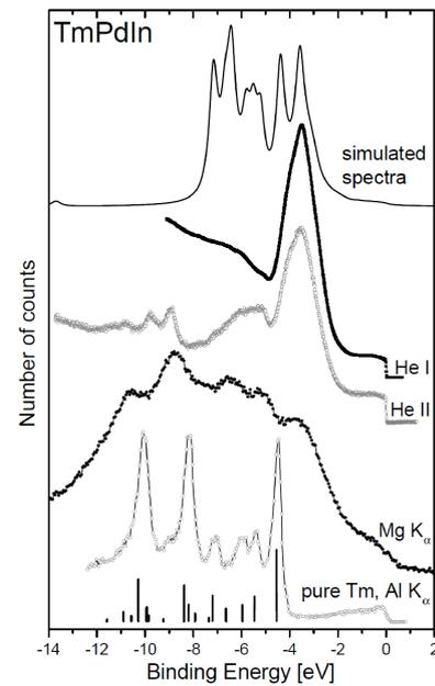
Fig. 3. Valence band of TmPdIn measured with He(I), He(II) (UPS) and Mg  $K_{\alpha}$  (XPS) radiation at  $T = 14$  K. The spectrum for pure Tm obtained with Al  $K_{\alpha}$  radiation from [11] is shown for comparison. Bars denote positions and intensities of the calculated peaks [11]. The uppermost curve is the XPS spectrum simulation from Fig. 2.
