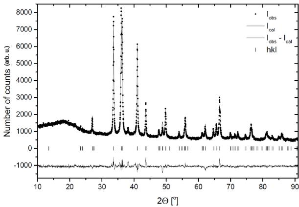
Fig. 1. X-ray diffraction pattern obtained for TmPdIn with Cu  $K_{\alpha}$  radiation at room temperature. Experimental data are marked with black points, solid line denotes a result of Rietveld analysis.
