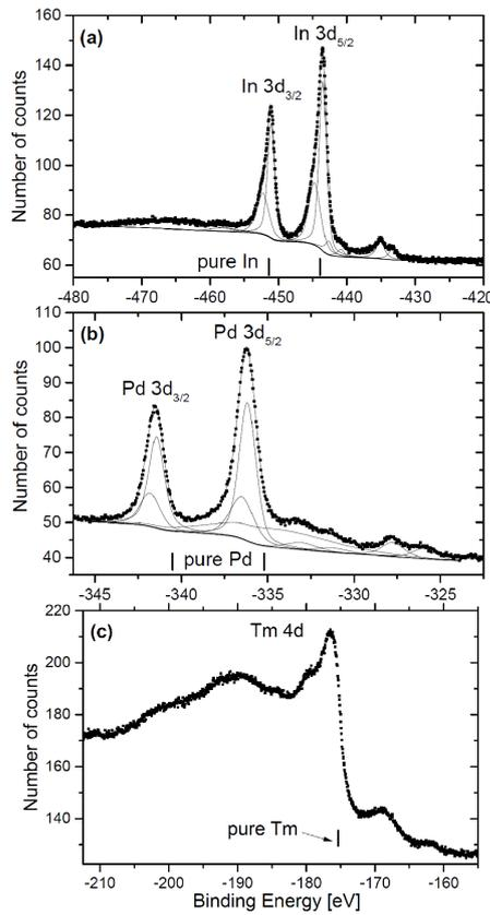
Fig. 4. XPS spectra for TmPdIn obtained with Mg  $K_{\alpha}$  radiation. Spectra for In 3d (a), Pd 3d (b) and Tm 4d (c) are shown. Binding energies for pure In, Pd and Tm are shown.
