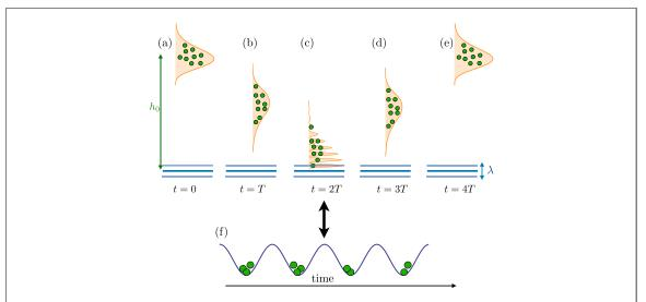
**Figure 1.** Setup figure of bouncing atoms on an oscillating mirror with period T for an n: 1 resonant driving where n=4. (a) The initially prepared atomic distribution at the classical turning point  $h_0$  returns to the starting position at t=4T (e). Figures (b)–(d) show the atomic distribution for time t=T, t=2T and t=3T, respectively. (f) In the effective description, the system is described by Bose–Hubbard model, see (4).
