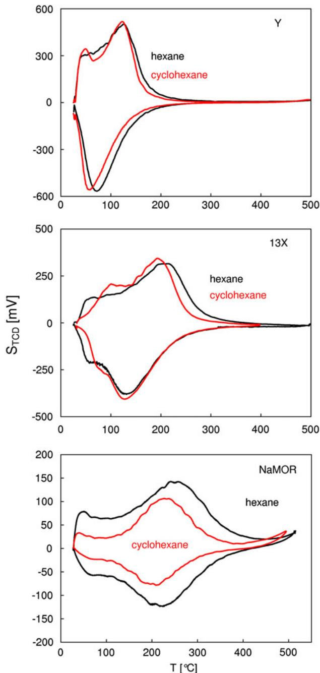
**Fig. 2** QE-TPDA profiles of hexane and cyclohexane on zeolites 13X, Y and NaMOR, measured at 10 °C/min. For 13X and Y partial pressures of hexane and cyclohexane equal to 6 and 7 mbar, respectively. For NaMOR they were equal to 8 and 6 mbar, respectively
