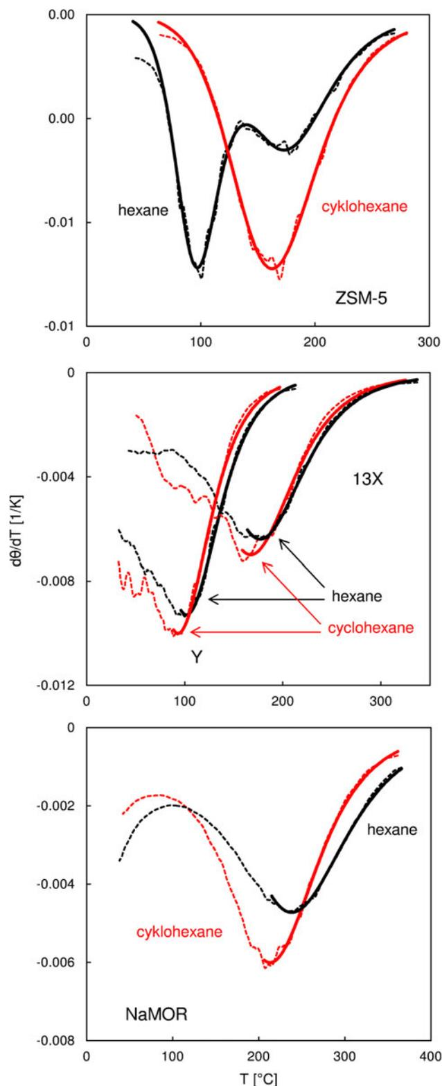
**Fig. 3** Fitting of the Langmuir and the DSL functions (solid lines) to the temperature derivatives of the normalized isobars determined by integration of the QE-TPDA profiles of hexane and cyclohexane (dashed lines)
