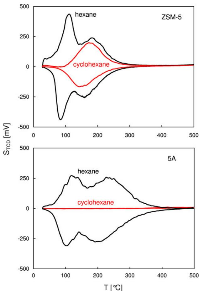
**Fig. 1** QE-TPDA profiles of hexane and cyclohexane on zeolites ZSM-5 and 5A, measured at 10 °C/min. Partial pressures of hexane and cyclohexane in the carrier gas equal to 6 and 7 mbar, respectively
