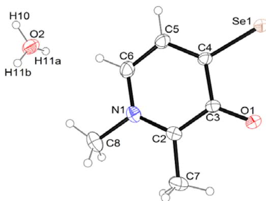
**Figure 4.** The asymmetric unit of 3-HDPSe-DIM with atom numbering scheme (displacement ellipsoids are drawn at the 50% probability level).
