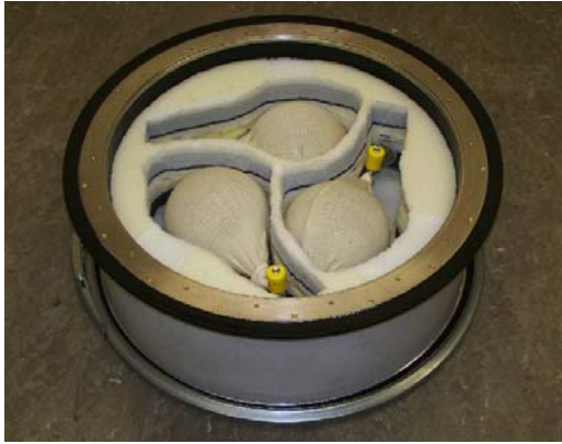
Fig. 5. Transport box and vessels from Mainz University group for ^3\text{He} storage during journey to hospital.
