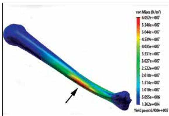
**Figure 4.** Distribution of stresses obtained from the 3 D model of humeral bone. Red color was used to mark the maximum stress of the humeral bone (arrow) taking into consideration forces of muscles given in Table 1.
