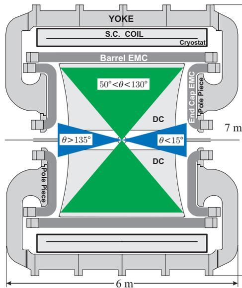
**Figure 1.** Schematic view of the KLOE detector.
