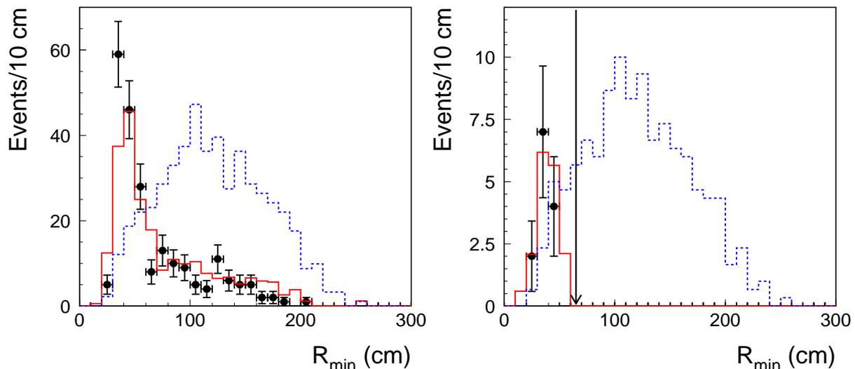
**Figure 7.** Distributions of  $R_{min}$  for six-photon events in the signal box applying the  $\chi^2_{fit} < 57.2$  cut (left), and applying  $\chi^2_{fit} < 57.2$  and  $\Delta E > 1.88$  cuts (right). Black points are data, background simulation is the red histogram. The dashed histogram represents simulated  $K_S \rightarrow 3\pi^0$  events.
