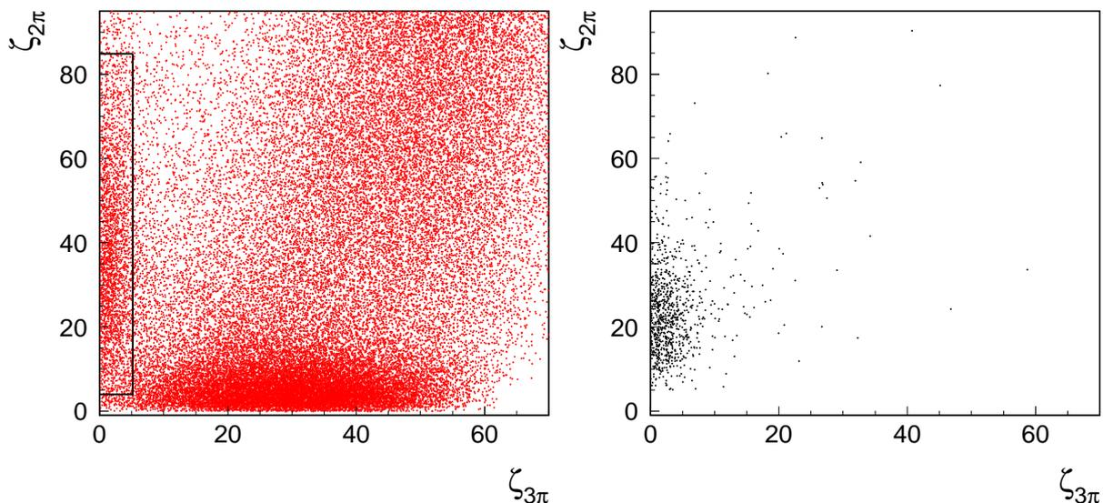
**Figure 4.** Distributions of events in the  $\zeta_{3\pi}$ - $\zeta_{2\pi}$  plane, for six-photon sample tagged by  $K_L$ -crash for data (left), and for the simulated  $K_S \rightarrow 3\pi^0$  decays (right). The solid lines show the signal region definition chosen using the optimization procedure described in the text.
