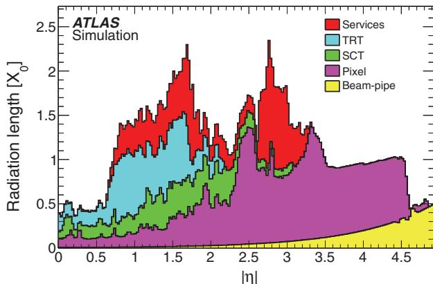
**Fig. 1** Amount of material in front of the cryostat, housing the solenoid and the EM calorimeters, in units of radiation length  $X_0$ , traversed by a particle as a function of  $|\eta|$ . The contributions of the different detector elements, including the services, are shown separately by *filled colour areas*
