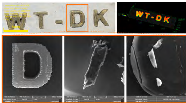
Fig. 7. 3D printouts obtained by exposing to laser source of light composition BI-PH-5B (0.1 wt%) + IOD (1.0 wt%) + mixture of monomers: CADE/TMPTMA (1/1 wt.). The top row contains images obtained from an optical microscope, while the bottom row contains images of the morphology of the "D" element of the printout, obtained using SEM (the scale bar represents left: 1 mm; middle and right: 10 \mu m) from SE (left and middle) and BSE (right) signal.
