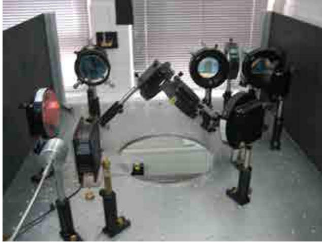
Figure 8.2: Optical system mounted at the top of the ^{129}\text{Xe} polarizer. It is enclosed in the box during operation for eye protection.
