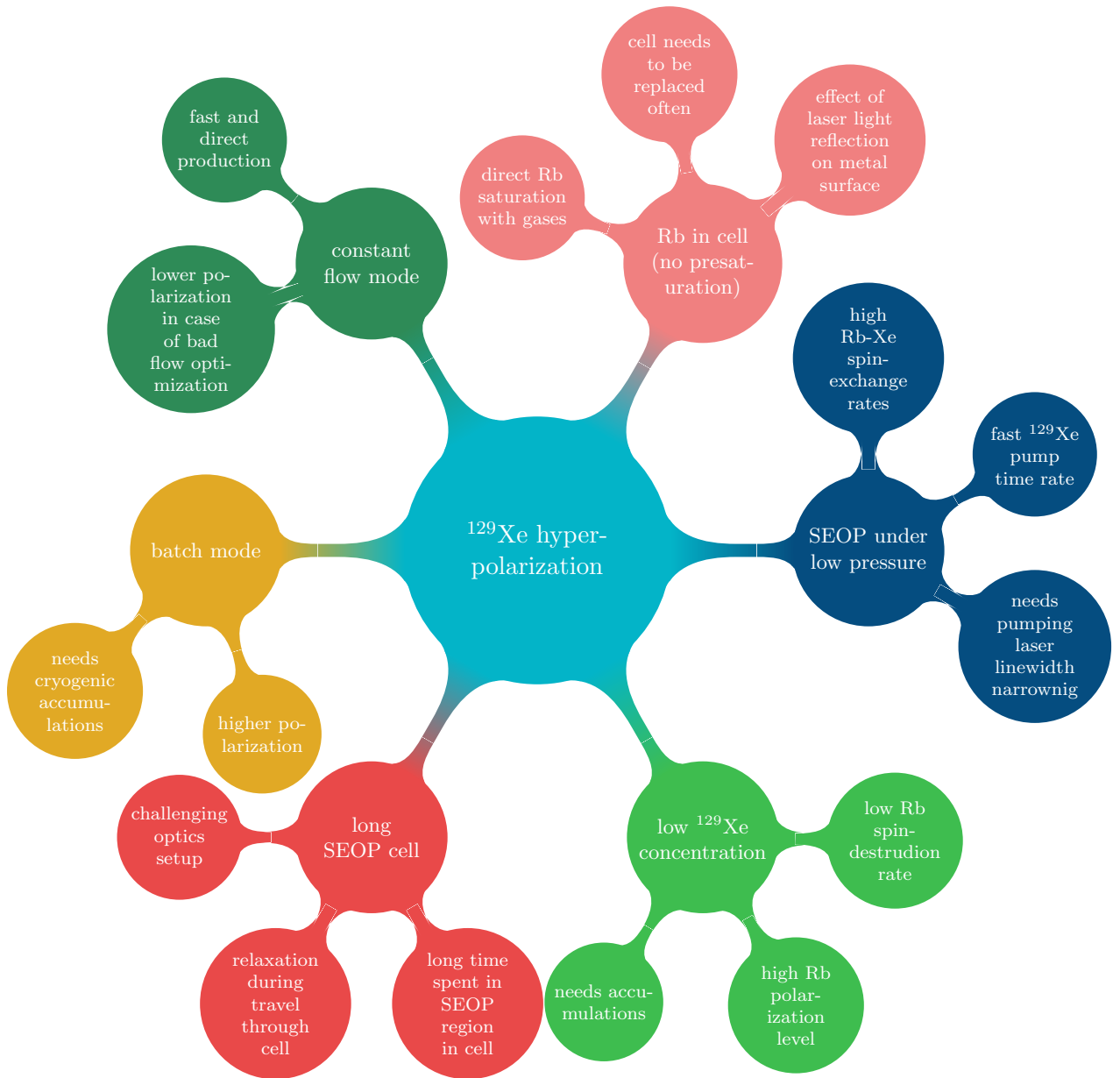
Figure 5.15: Summary of favorable and unwanted processes during the SEOP experiment for polarizers operating at \sim 1 bar pressure, low ^{129}\text{Xe} concentration and large volume SEOP cell.
