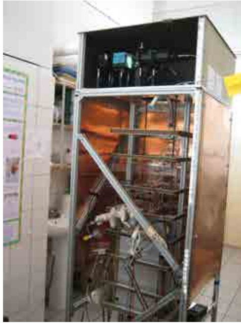
Figure 4.9: Overall view of the xenon polarizer. Four copper sheets are mounted on aluminum profiles form a Faraday cage (one wall was removed for closer look inside). The optical setup can be seen at the top, also enclosed during operation.
