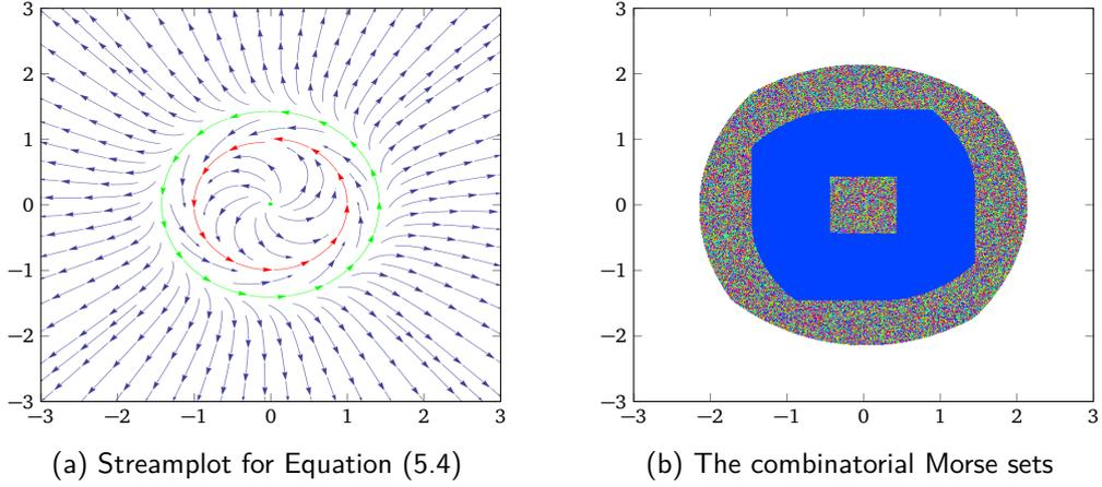
FIGURE 5.2: Visualization of the flow from Equation (5.4) for  $\mu = 2$  in  $M = [-3, 3] \times [-3, 3]$  and outputs when using the fixed time step  $h = 0.0006$  as described in Section 5.4.1. There are 57673 spurious combinatorial Morse sets. Most of them consist of just one box. Calculating the Morse graph was impossible because of memory problems.
